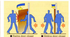
The sliding door closer system eliminates dead space and ensures high safety.
